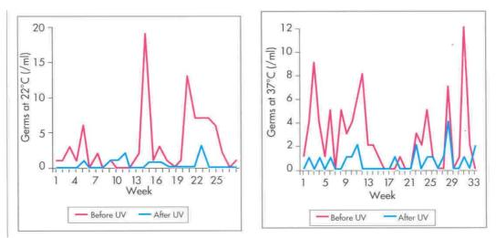
figure 6 : Disinfection results of the system  $ClO_2/UV$  for HPC (Esparza, 1997).
